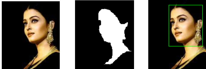
Figure 2.2: Example of skin color segmentation for face detection (Tripathi, et al, 2011, 7)
