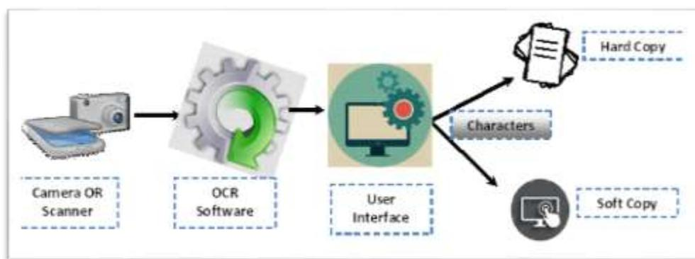
**Figure 1 Logical Component of OCR System**
