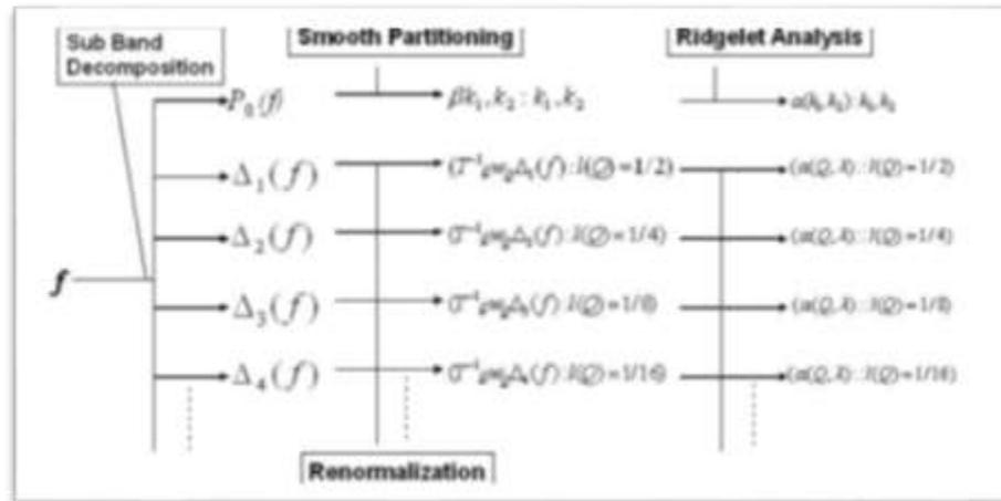
Figure 8 Overview of Curvelet Transform scheme (Majumdar, et.al., 2007)
