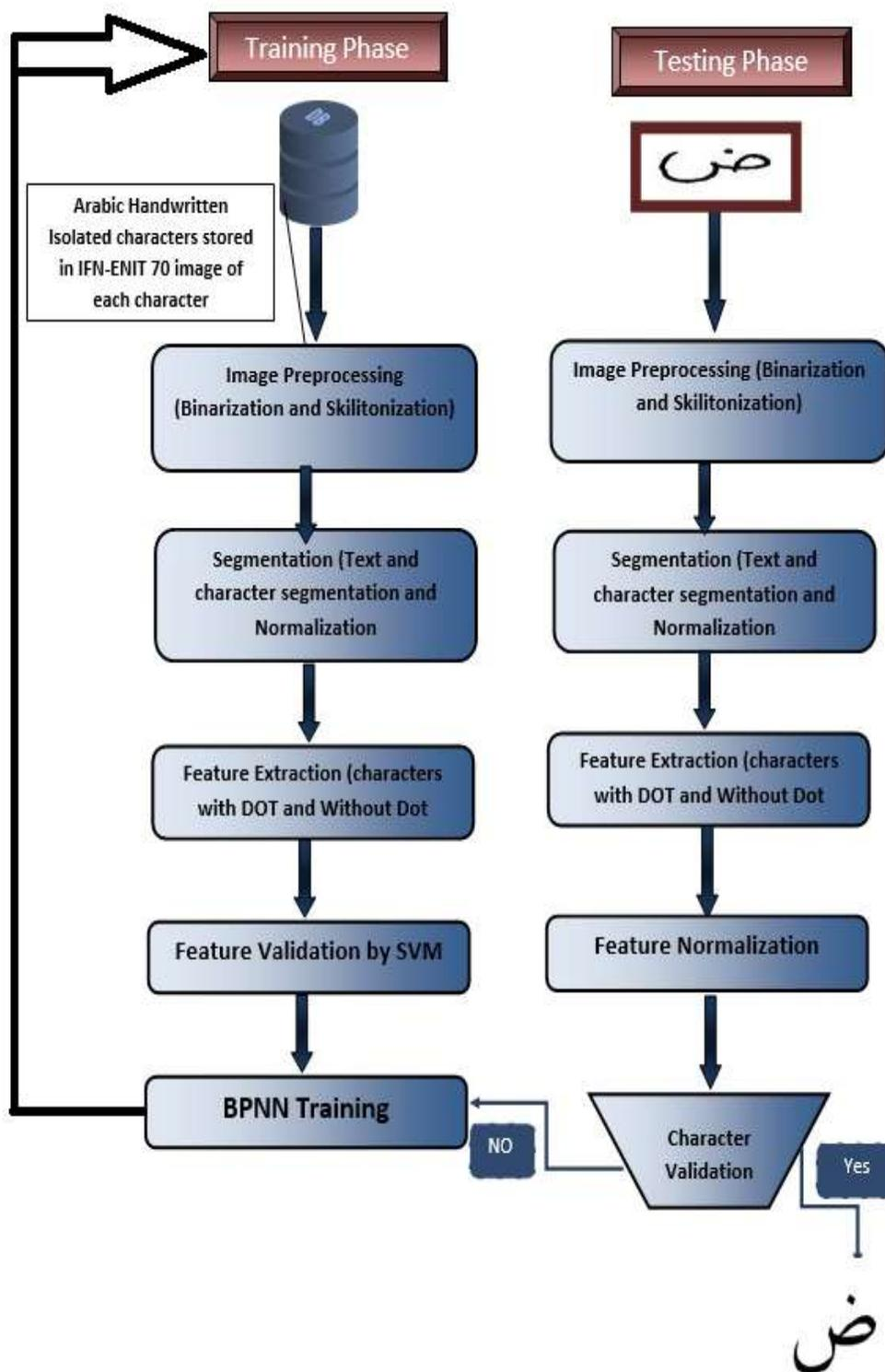
Figure 11 OCR Block Diagram
