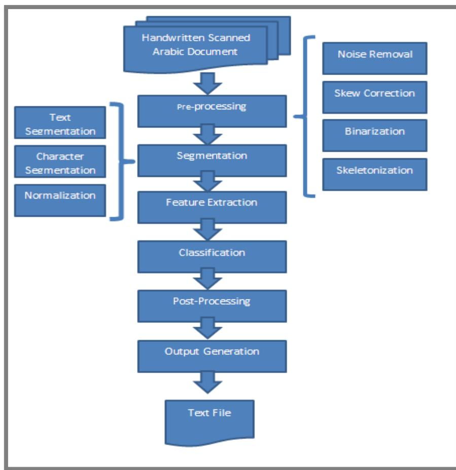
**Figure 2 AHCR System's General Structure**
