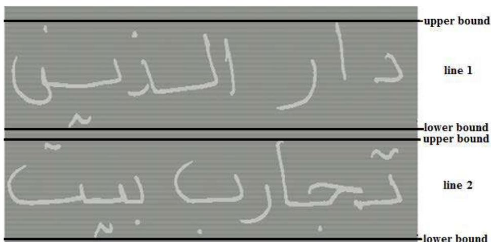
**Figure 16 Line segmentation model: Source (Al-Ani, et.al., 2014)**
