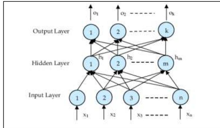
**Figure 13 Basic Block of Back propagation neural network**
