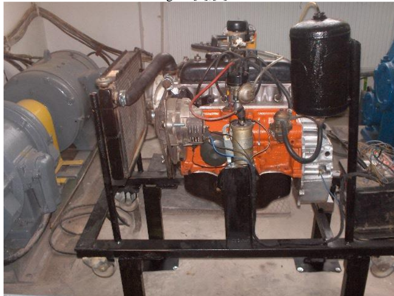
Fig.1 Experimental bench to measure the temperature values of ICE. In ICE heat produced during operation is transferred to a lesser extent during the gas engine fluid change.
