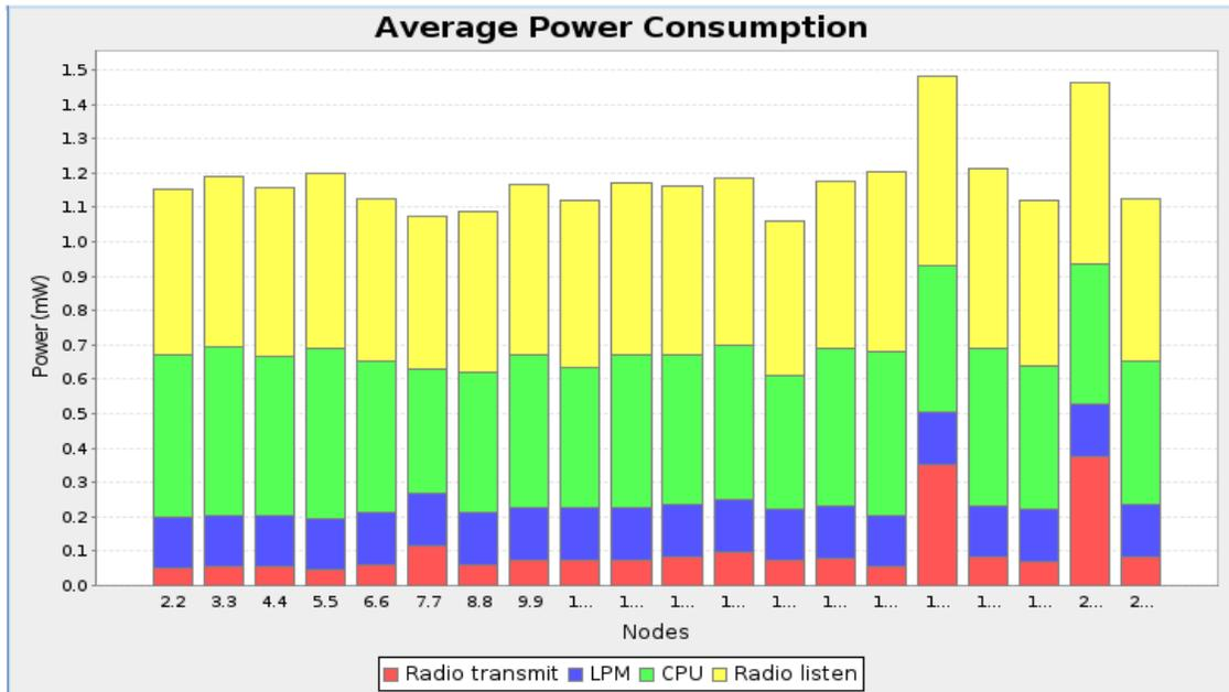
Figures 4-10 power consumption when RX RATIO 100%
