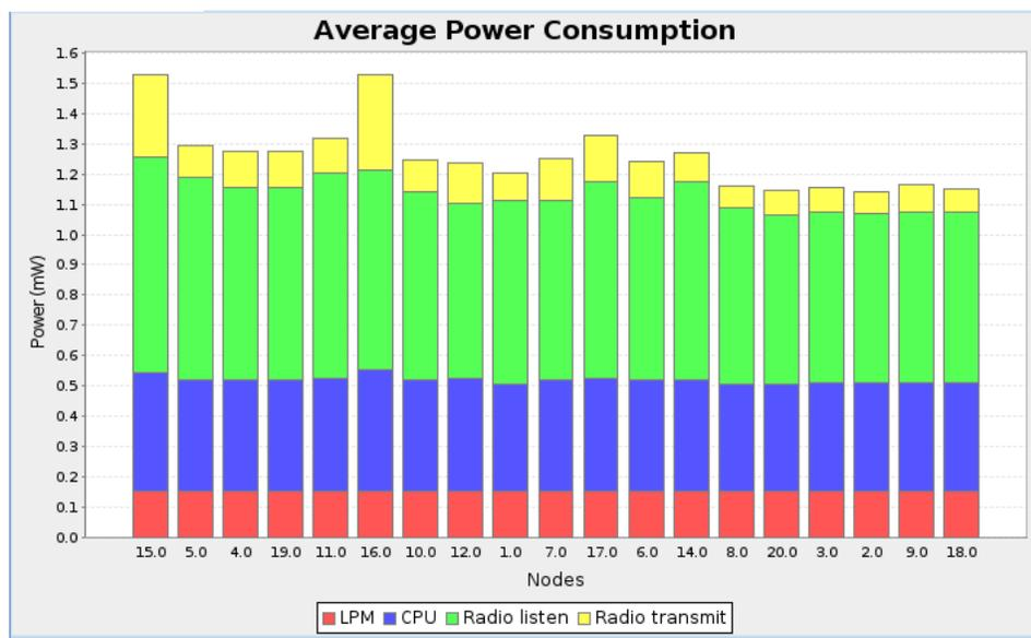
Figures 4-5 power consumption when RX RATIO 100%
