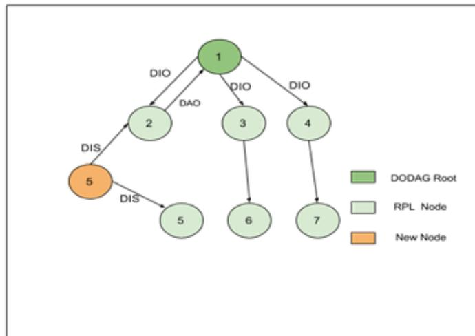
Figure 2.4 A Typical DODAG (Cisco Systems,2012)
