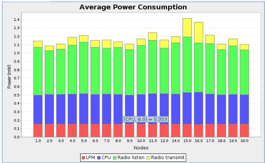
Figures 4-6 power consumption when RX RATIO 80%
